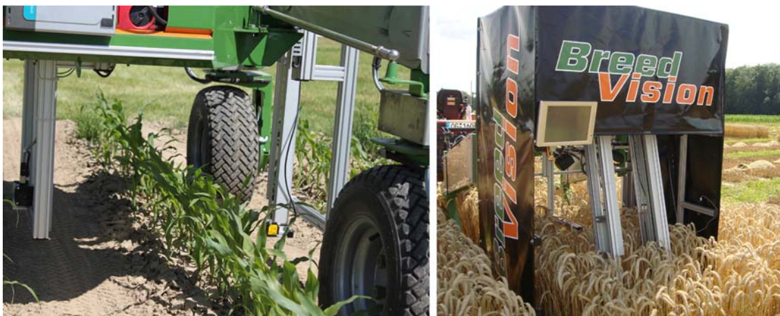
Figure 1 Sensor integration into the phenotyping-platforms “BoniRob”(left) and “BreedVision” Plants having structures smaller than the spatial resolution of the applied sensors and with plant coverage densities which avoid a redetection of single plants with available instruments
